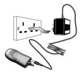
To charge the transmitter using the QT424/1 charger, simply connect the charger to a standard 13A mains socket and to the 1.3mm socket located next to the transmitter's pull-clip as shown (right). To charge using the QT424/10 charger, please refer to the separate instructions supplied with the charger.
